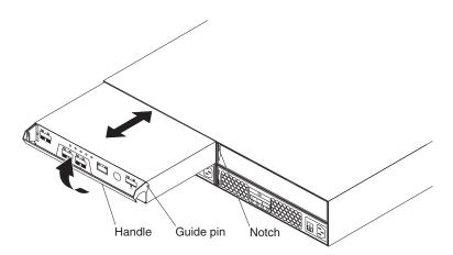
Figure 39. Installing a controller
